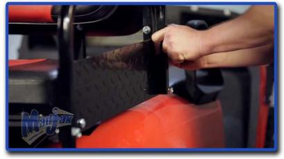
Attach the two back bolts to the armrest. Once all bolts are in place you can tighten hardware.
