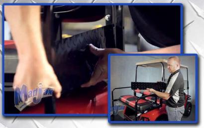
Once the nut from the front bolt and the back two bolts have been removed. Make sure the diamond plate faces outwards and place the side panel between armrest and seat frame.
