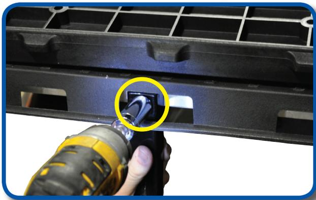
Attach bagwell bracket to polyboard seat frame as shown using hardware from pack 2. Repeat process on other side.
