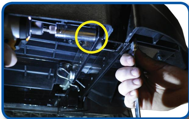
Attach grab bar to footrest as shown using 10mm hardware from pack 6.
