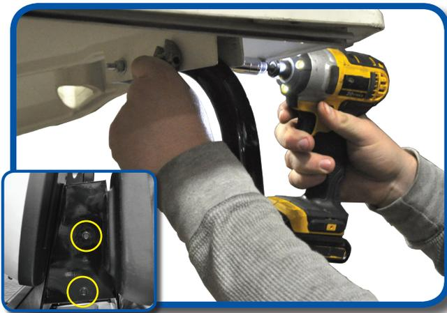
Re-attach roof using hardware retained from Step 1 as shown. Attach struts to main bracket using hardware from pack 8.
