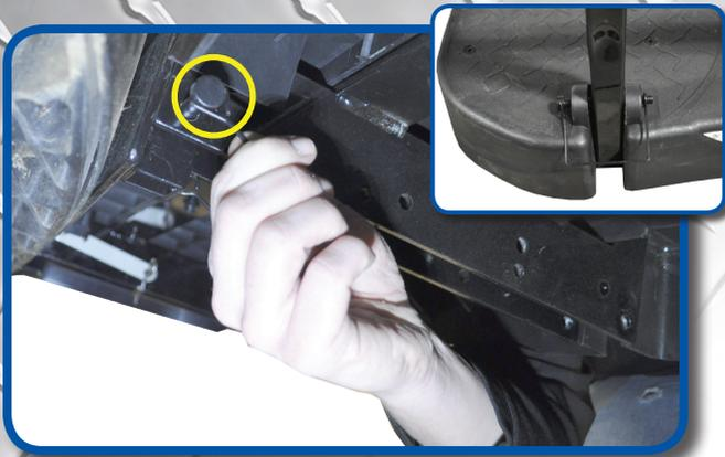
Using quick release clips from hardware pack 6 Secure footplate to bagwell bracket and grab bar as shown.
