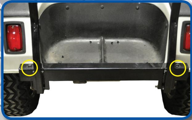
Attach bagwell bracket to frame as shown using hardware from pack 2 and tighten.
