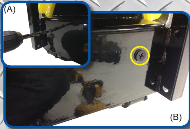
A) Using a 3/8" Drill bit, drill through bumper into bagwell.
