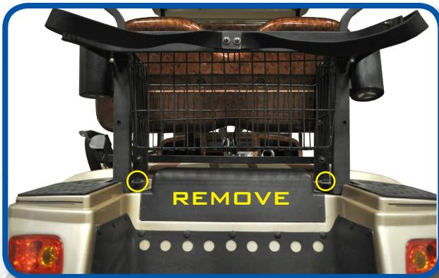
Remove basket by removing hardware located inside motor compartment. Retain factory hardware.
