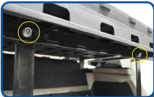
Attach seat frame to bagwell brackets using hardware Pack 2.
