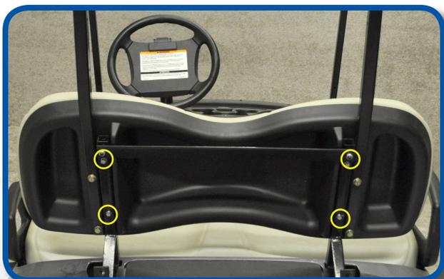
Cut plastic divider in bagwell if required. Remove factory bolts from bagwell. Enlarge hole by drilling using a 7/16" drill bit.
