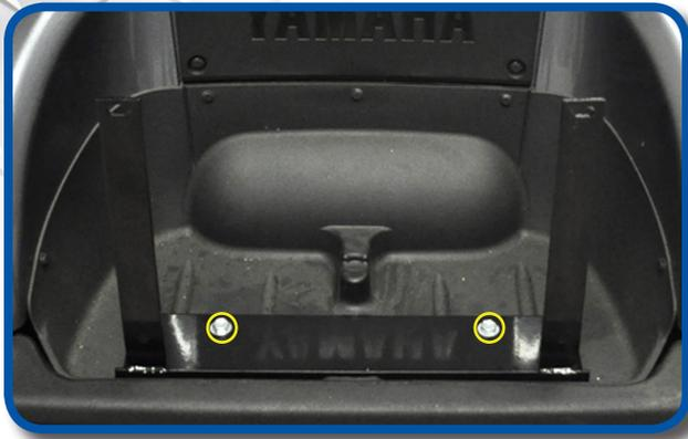
Attach bagwell bracket using hardware from Pack 2.
