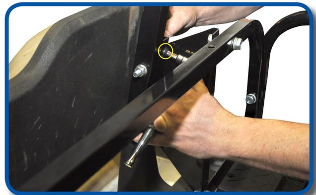
1. Place HD bracket on flip seat as shown. Align bracket holes to the flip seat mounting holes.
