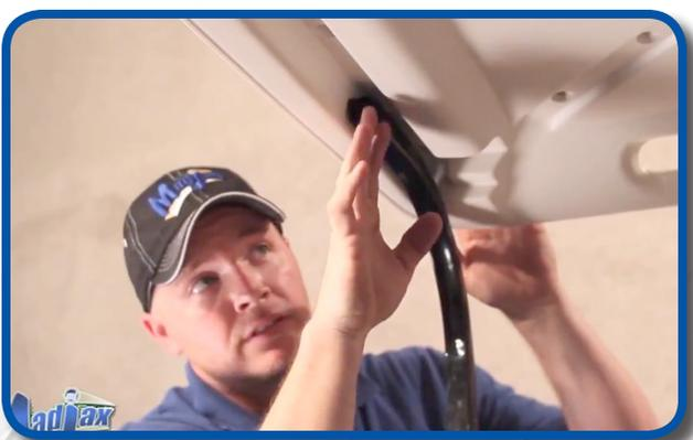
After rear struts are attached, remove brace. Insert rear struts into canopy channel. Using hardware retained from Step 1, attach rear struts to the canopy.
