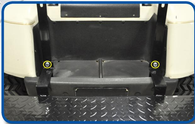
Attach footrest as shown using remaining hardware from Pack 3.
