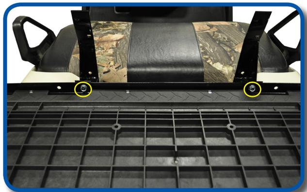
Attach rear seat frame. Using hardware from Pack 3, attach to the front lean back brackets.
