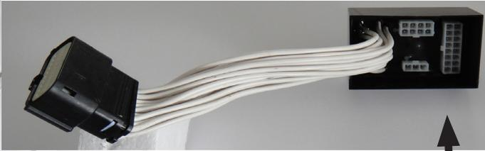
NOTE: Module shown is for the Club Car Precedent, DS and the \*E-Z-GO® TXT® 48V, for Connector location for other Vehicles see the installation instructions for the specific Vehicle.
