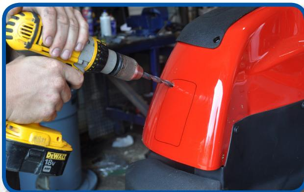
Drill a pilot hole and cut, again staying to the **INSIDE** or on the mark.
