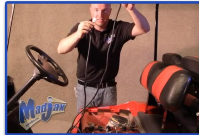
\*Make sure cart is in TOW mode. Feed front harness down through the front of the battery component. Run short tail light wire under the seat and over the tire well on the drivers side.
