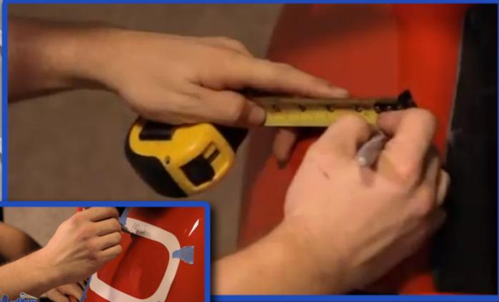
Using the measurements provided on your tail light template, measure and mark your template. Use a marking pen to trace the inside line. \*Flip template over to use on other side.
