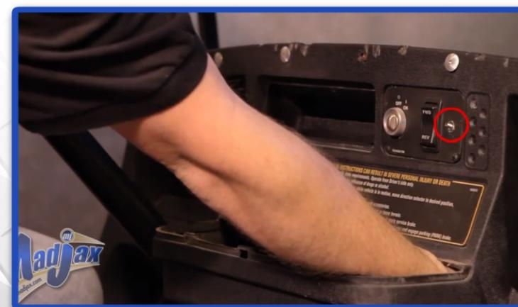
Remove cup holder. Feed threaded end of switch through the dash where the hole was drilled. Retain hardware\*
