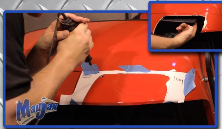
Cut out the shape of the headlight. \*Use the cutting tool to remove the excess trim. Keep your template for the other side.
