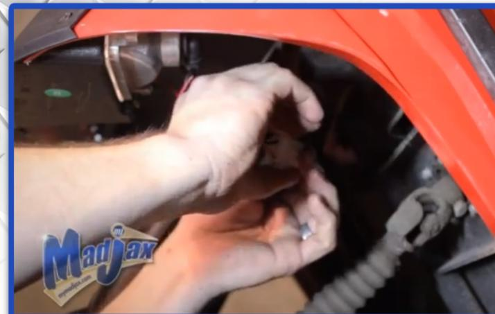
Attach front headlights to wire harness. Secure excess wire with zip ties.
