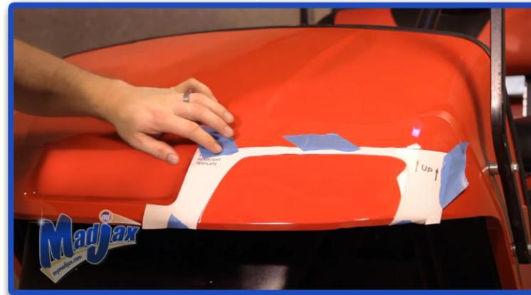
Drill pilot hole on the inside of the template line.
