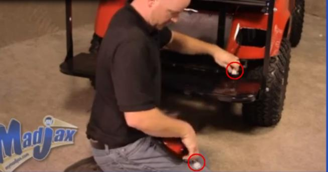
Attach rear tail light wire harness. Then place tail light into the rear of the vehicle. Insert four screws into tail light using supplied hardware. Secure wire with ties. \*Repeat process on other side.
