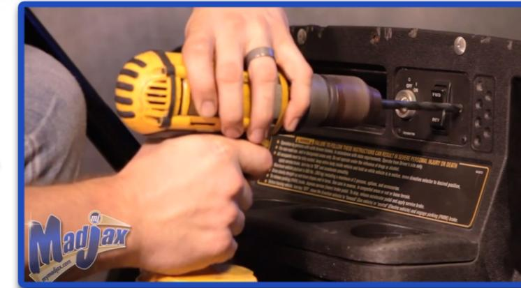
Run the wire harness through the holes under the frame to secure the harness. \*Use the zip ties provided.
