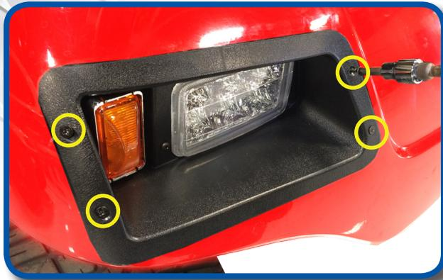
Place headlight assemblies into cutouts and attach to wiring harness. Fasten headlight assemblies to cowling using the supplied screws. **IMPORTANT: DO NOT OVERTIGHTEN SCREWS.**
