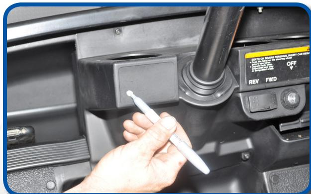
Locate a place on the dashboard to mount the switch. We recommend using the location shown as it does not interfere with the cup holder when reinstalled and also allows you to easily route the wiring harness.
