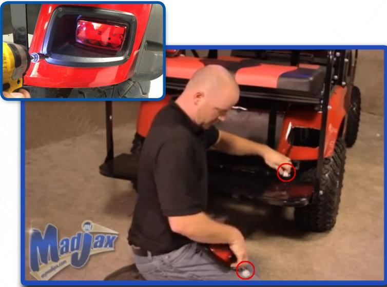
Attach rear tail light wire harness. Then place tail light into the rear of the vehicle. Insert four screws into tail light using supplied hardware. Secure wire with ties. \*Repeat process on other side.
