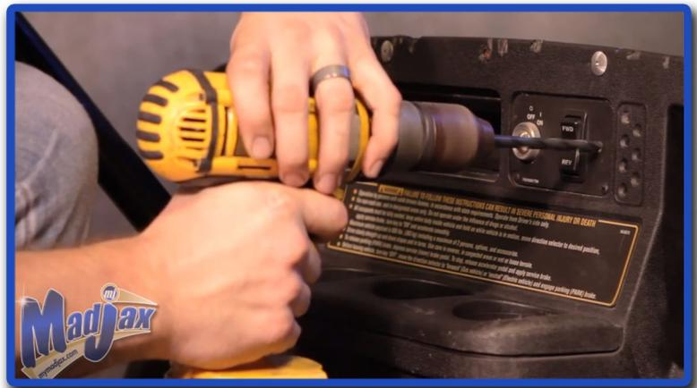
14 Remove cup holder. Feed threaded end of switch through the dash where the hole was drilled. Retain hardware\*
