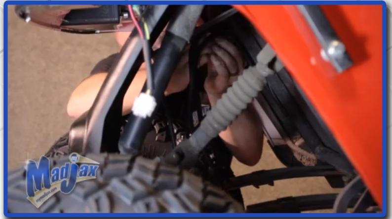
12 Attach front headlights to wire harness. Secure excess wire with zip ties.
