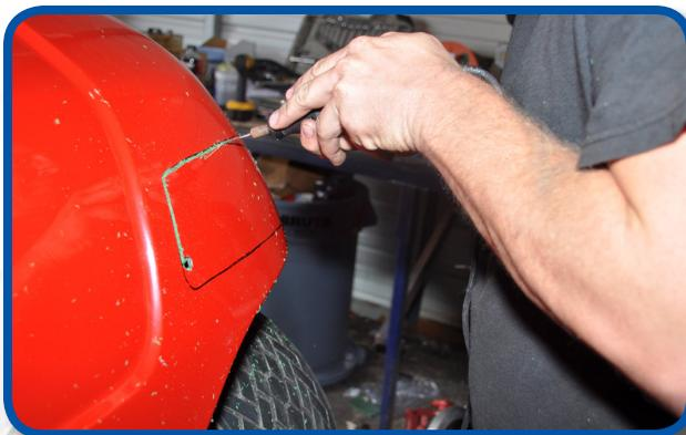
Cut out bodywork. **IMPORTANT:** As you approach the top of the cut, back out the cutting tool to prevent cutting into the fender well. Cut the cowling to the inside of the mark.
