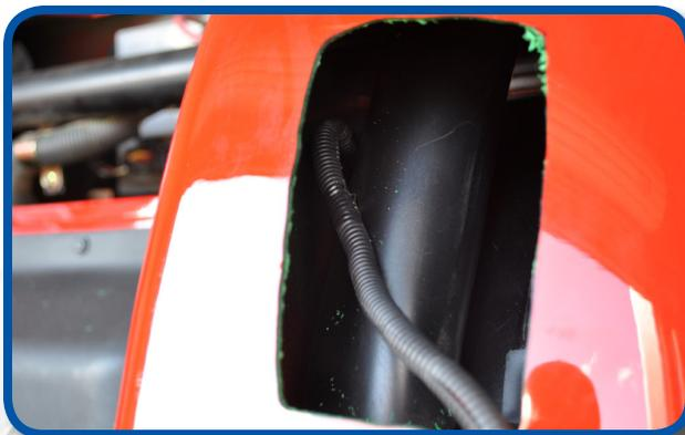
Route wiring harness behind rear fender wells. Attach rear lights and mount to bodywork using supplied screws.
