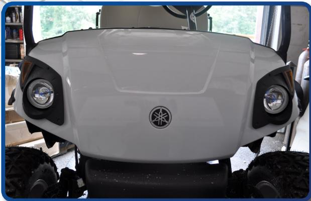
Place headlight assemblies into cutouts and attach to wiring harness. Fasten headlight assemblies to cowling using the supplied fasteners.
