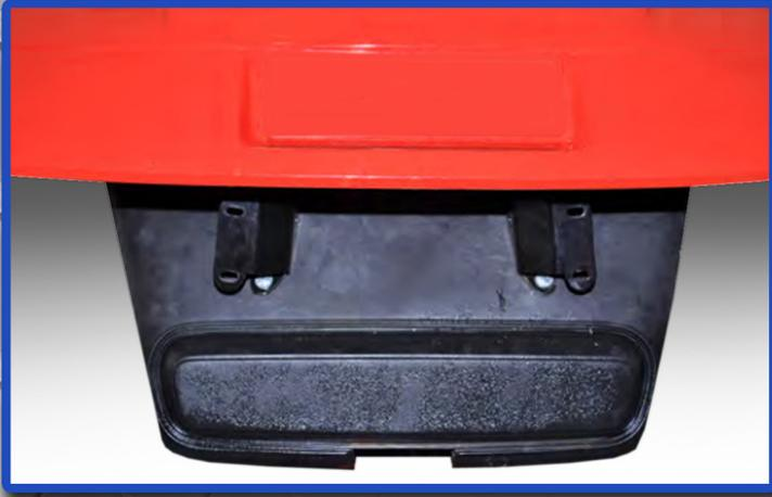
Install mounting brackets with mounting holes facing out using hardware retained from step 1.
