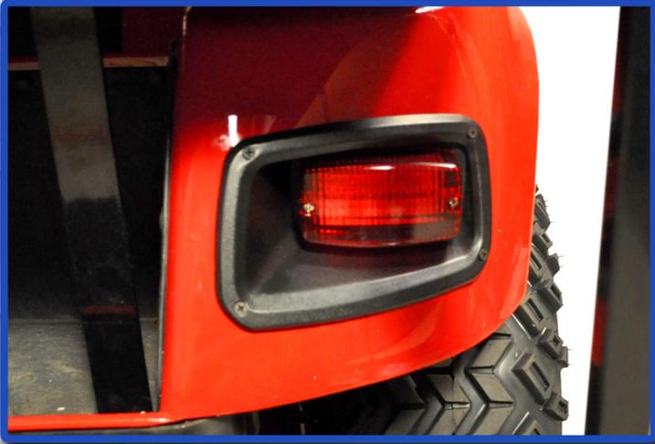
Attach tail light to harness, then insert tail light and attach tail light to cart using provided hardware. Connect red connector on harness to passenger side lights and white connector to driver's side lights.
