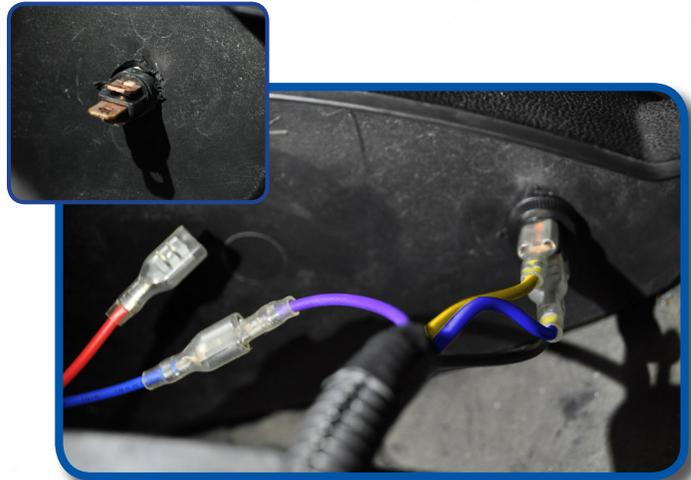
Attach horn to purple and black female spade connectors and secure horn under front cowl.
