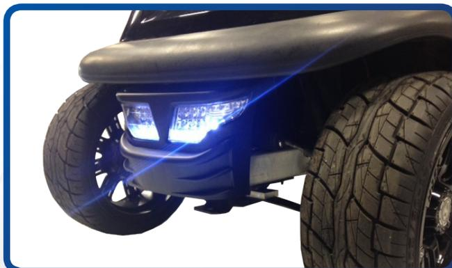
When you turn on the key switch the daytime run lights will now come on. They will stay on when you turn on the headlights and will only turn off when the keyswitch is off.
