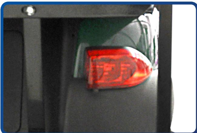
Using a wire snake, pull the tail light connector through the hole in the rear body. Connect the tail lights to the vehicle tail light wiring harness. Determine the desired location of the tail lights. Remove the double sided tape from the back of the tail light and mount to the rear body using eight screws provided.
