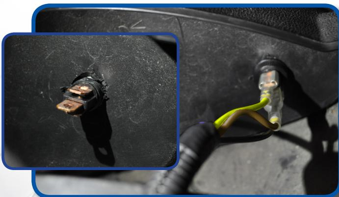
Route the 6 pin headlight connector through the cutout in the passenger dash. Plug the 6 pin male wire harness connector into the 6 pin female headlight wire harness connector and wire tie harness to frame support (the two extra wires on this harness are for use with the optional horn kit).
