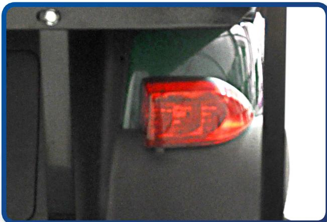
Using a wire snake, pull the tail light connector through the hole in the rear body. Connect the tail lights to the vehicle tail light wiring harness. Determine the desired location of the tail lights. Remove the double sided tape from the back of the tail light and mount to the rear body.
