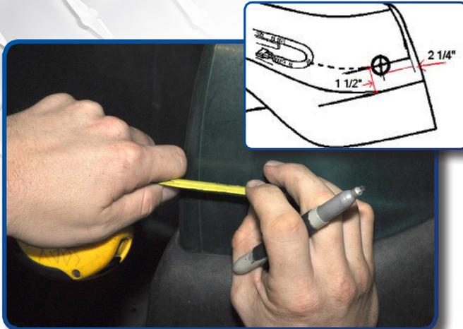
Before removing double sided tape and installing the LED Tail Lights, test fit them in their position on the rear location of the vehicle. Mark the center of the tail light hole using drawing Using a 1-1/2 inch hole saw, drill a hole in the location as shown in drawing 1 . Sand to remove sharp edges.
