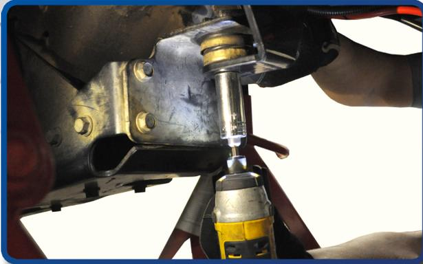
Carefully lower the jack until the bolt threads extend through the small hole on the new engine mount bracket. Tighten the bolt and hardware using the 15mm socket.
