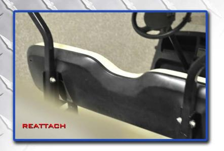
Reattach seatback using hardware from step 2.
