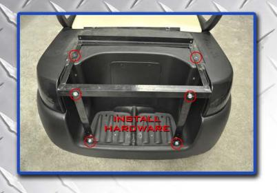
Attach mounting bracket to golf cart using hardware from step 6.
