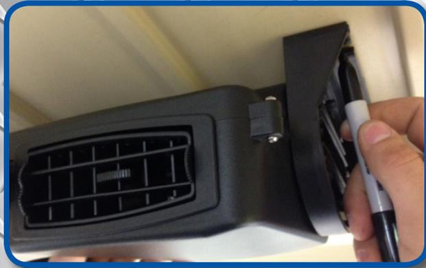
With the help of an assistant mark the desired location you want to mount the fan. Use a tape measure to square the brackets to ensure proper alignment.
