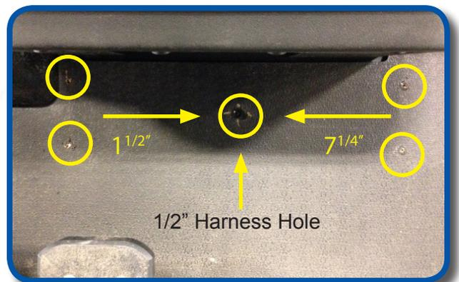
Attach fan to floor using four 6mm x 45mm hex head bolts as shown. Use rubber side of washer at fan bracket and underneath cart to seal hole. Once all 4 bolts are in place, tighten hardware. Route harness under cart to battery compartment and secure to frame using supplied zip ties. See STEP 9 for In-Line fuse instructions.
