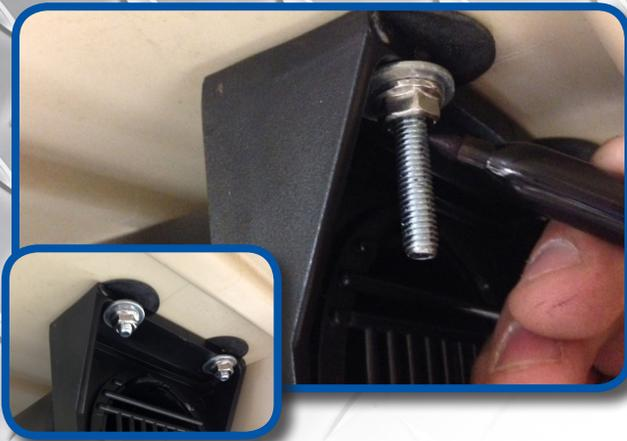
Trim off excess bolt by marking threads. Remove and cut one bolt at a time using a hacksaw.
